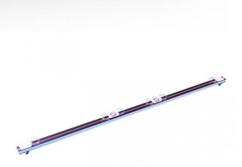
This track is an excellent alternative to conventional air tracks. In fact, the natural friction of moving mobiles is greatly reduced by magnetic levitation of the mobiles.
