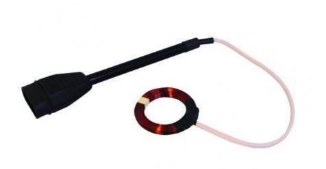
Power the coil, then approach it with a straight magnet. The coil is put on the magnet and positioned in the centre, so that the flow entering the south face is then at its maximum.
