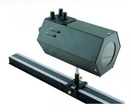
Aluminium case equipped with 3 LEDs of very bright primary colours, to study colour mixtures. Potentiometers independently control the light intensity of each of the LEDs, until they are turned off. We thus obtain three coloured disks that intersect: formation of secondary colours and white in the centre. The print also allows you to have a large white surface to achieve the subtraction of the colours with the use of a ball on a rod (not provided).
