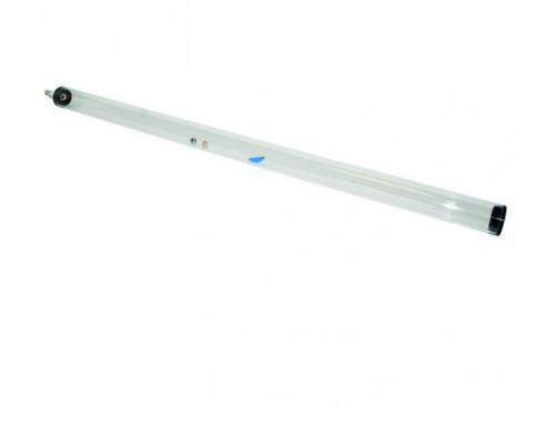
Vacuum tube to demonstrate that the acceleration and the fall time are identical for all bodies in a vacuum, in the absence of air resistance and vertical thrust.
