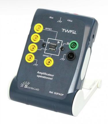
This stand for an operational amplifier consists of an insulating housing on which is fixed an 8-pin integrated circuit support.
