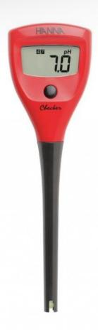
Light and compact pH meter tester , ideal for accurate and fast routine measurements. It has a narrow electrode, ideal for test tube measurements. With 2-point calibration, it provides measurements with an accuracy of  $\pm$  0.2 pH. The pH electrode with S7 connection is easy to replace.
