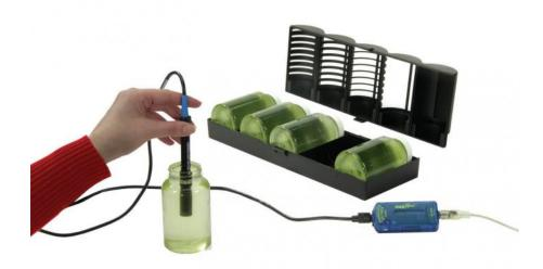
This study system allows a reliable and repetitive measurement of photosynthetic intensity as a function of light intensity. Consisting of 5 250ml plastic bottles and a plastic stand, this system allows a very precise control of the amount of light received in each container and allows accurate analysis.
