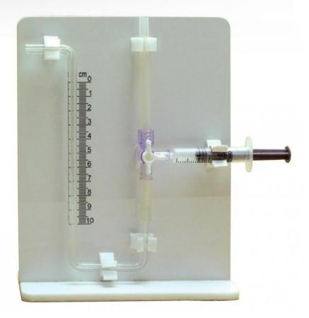
This device allows easy and effective measurement of plant transpiration. This potometer, compared to other models, is very resistant because just one component is glass (capillary tube) which limits the risk of breakage.
