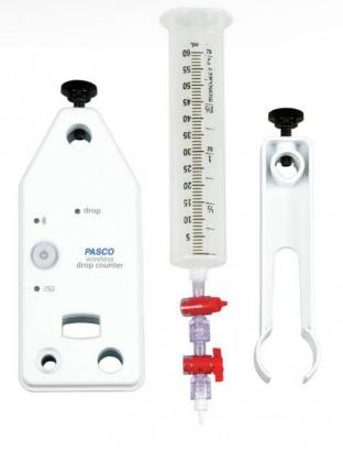
Add the wireless drop counter for more efficient and accurate titration data. This wireless sensor counts the drops of reagent added during titration and converts them into volume. Use with a wireless pH sensor, wireless temperature sensor, or wireless conductivity sensor to easily perform pH-metric, thermometric, and conductivity titrations.
