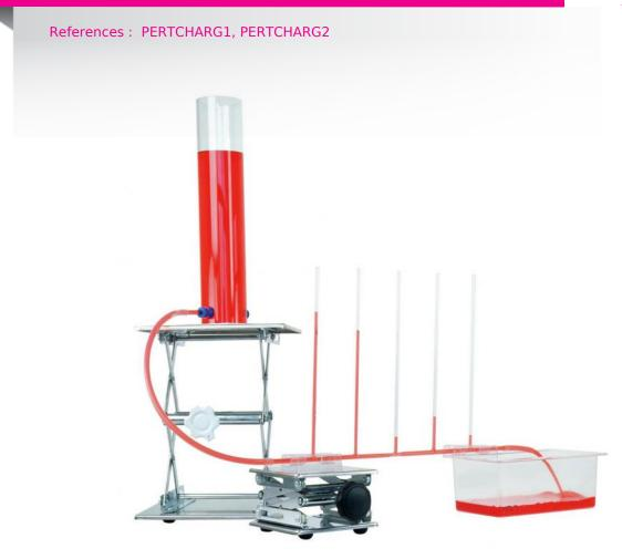
Models designed to study the pressure along a constant or variable diameter tube through which a liquid flows. Manometric tubes are placed along the flow tube.
