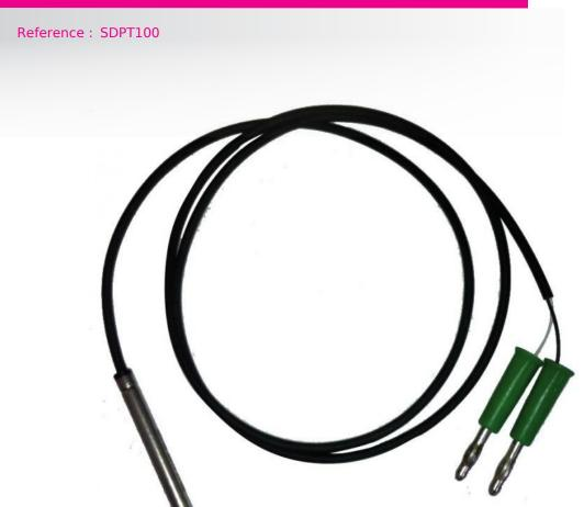
Pt100 probe, output on Ø 4 mm banana sockets Platinum resistance device (Pt) which has the characteristic of having a resistance of 100  $\Omega$  at 0 ° C. Its resistance varies according to the temperature.
