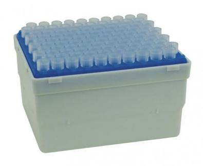
Rack of 10-200  $\mu$ l yellow cones Cones presented in a 96-point rack. Polypropylene rack with transparent polycarbonate lid. Autoclavable at 110° C.
