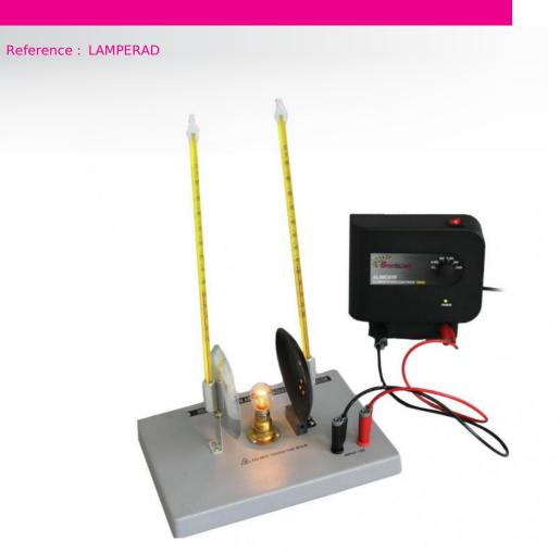
Device for showing the transfer of light energy from a hot lamp.
