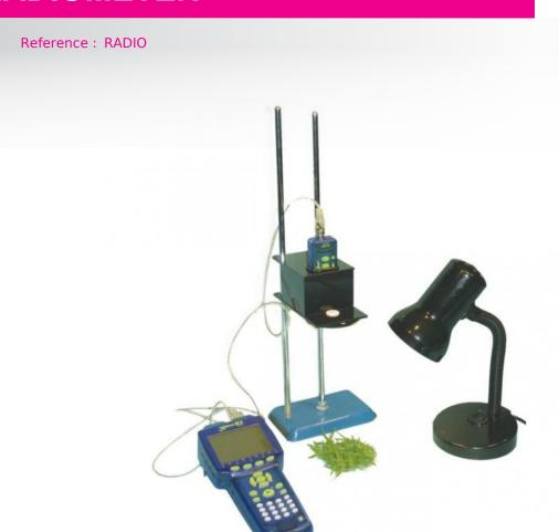
The radiometer is a device that makes it possible to determine the spectral properties of materials.
