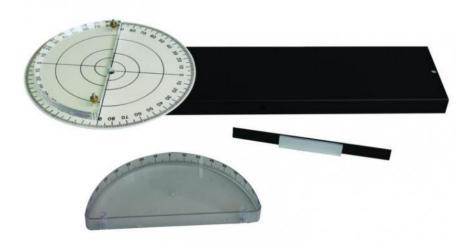
This complete set allows the study of reflection and refraction without an optical bench. It is composed of a sheet metal support on which is fixed a 230 mm diameter graduated disc, a 200 mm diameter hemi-cylindrical tank and lens, and a plane mirror mounted on a magnetic support. The set can be used in horizontal or vertical position: Ø 10mm rod included, to be completed by an optical stand.
