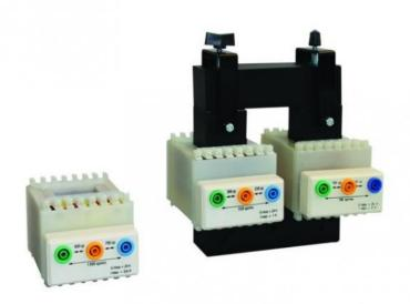
130 turn coil Intermediate sockets: 30 and 100 turns
