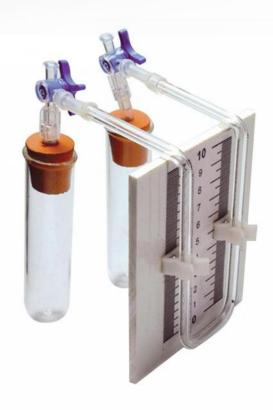
This device was designed to study the gas exchange resulting from the respiration of small organisms (meal worms, snails ...) or resulting from photosynthesis for a plant.
