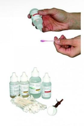
This kit can detect the presence of blood on fabric or other materials by performing a Kastle-Meyer test. A wet cotton swab is rubbed on the tissue to be analysed and the reagents are poured over it. The appearance of colour indicates the presence of human or animal blood. Positive control strips are used to verify that the technique is working and to obtain the control colour.
