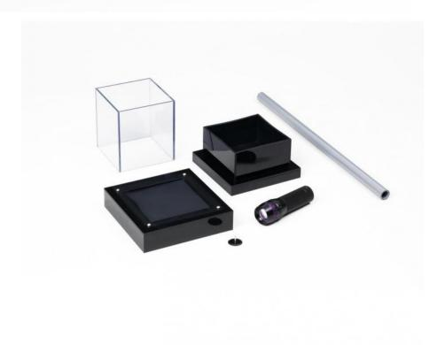
Cloud chamber requiring no current source or dry ice. It can be entirely assembled by students, making it educational. Just cool the base in the freezer, place ethanol on the top and fill the hot water tank. After a few minutes, the fog is formed and the first traces of the charged particles appear.
