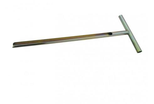
The wide opening of this soil sampler facilitates inspection of the soil sample while it is still in the auger. The total length of the sampler is 63 cm and gives a soil sample about 49 cm long and 22 mm in diameter. Made from galvanised iron.
