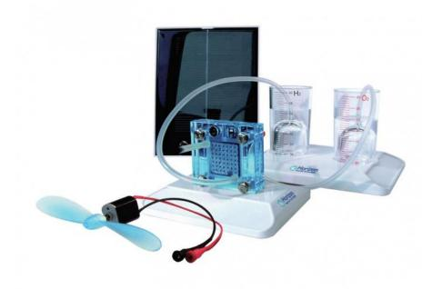
This set allows the transformation of solar energy into electrical energy through a reversible fuel cell. Included: Photovoltaic cell, fuel cell, hydrogen and oxygen tanks, motor with blades, connection cords and accessories, assembly and operating instructions.
