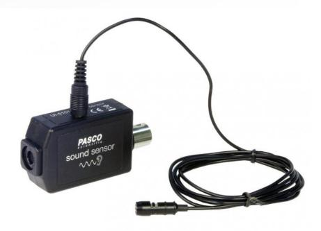
The sound sensor contains a sensitive microphone designed to measure the relative loudness of sound and display audio waveforms and sound levels between 45 and 100 dB when used with the 550 or 850 interfaces.
