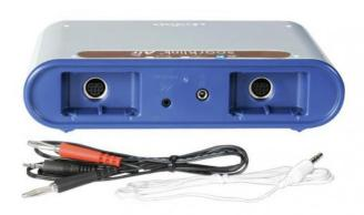
Connect the sensor of your choice and connect the interface via Bluetooth to the computer work station (a computer interface).
