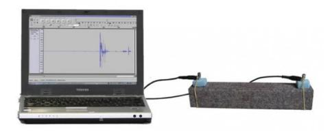
This kit makes it possible to measure the propagation velocities of seismic waves in different materials, it is accompanied by a very detailed note which suggests a PW session in two parts.
