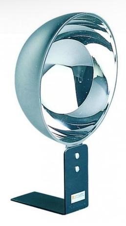
Plastic hemisphere covered on both sides with an aluminium layer, thus constituting a spherical mirror that is concave on the inside and convex on the outside. This mirror makes it possible to obtain real images of objects.
