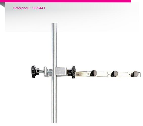
This stand allows you to simultaneously position 3 springs while being sure that they are exactly at the same height. The suspension points are spaced about 50 mm apart.
