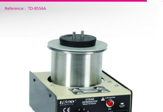
Hot steam is essential for most introductory experiments in thermodynamics. This steam generator is an inexpensive heat sink with a perfect constant temperature that generates a plentiful supply of steam. It brings 3/4 litre of water to boiling in 10 minutes and provides continuous steam up to 10 grams / min. Characteristics:
