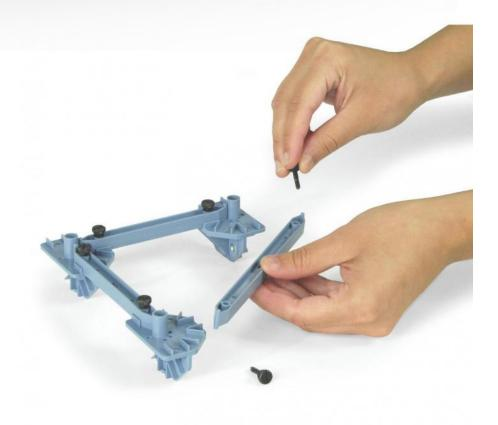
This kit will allow the construction a variety of different structures to study the trellis principles. The ABS plastic beams connect securely together using the knurled connectors and knurled screws provided. The strain gauges can be inserted anywhere in the structure by replacing beams. Weights (not supplied) can be hung from the structure to establish constraints.
