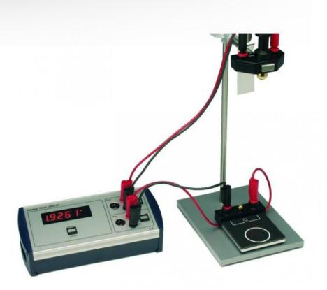
This device is designed for use with an electronic meter to determine the falling time of a free falling ball. The timer is triggered when the ball is released and stops when the ball comes into contact with the receiver board. The precision of the chronometer allows very realistic results.
