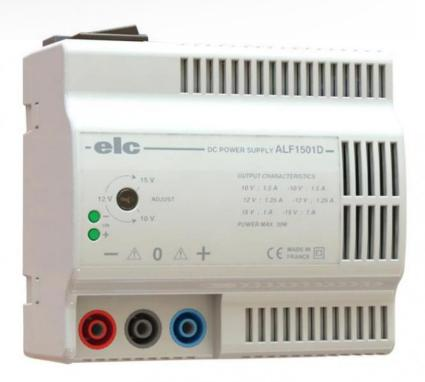
Symmetrical laboratory power supply with 0 Volts common to both outputs. Symmetrical output voltages: adjustable from  $\pm$  10 to  $\pm$  15 V linearly. Electrical connections with banana safety sockets Ø 4 mm
