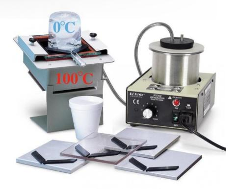
One of the most important features of buildings in the modern world is their ability to provide good thermal insulation. This device provides students with a way to observe and quantify heat flow. Students use 5 common materials glass, wood, polycarbonate, Isorel and plaster Operation:
