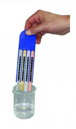
Device composed of an insulating support on which are fixed different metal blades of identical length. Each blade is equipped with a liquid crystal thermometer to display the temperature of the blade. Immersed in boiling water for example, it is possible to visualize the temperature rise of each blade without an additional thermometer
