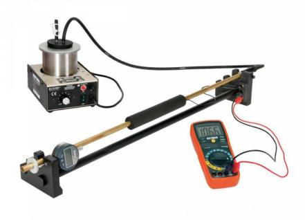
With the PASCO thermal expansion device, students can accurately and easily study the expansion of metals at increasing temperatures.
