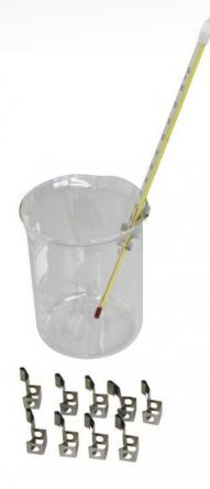
Supports attached to the edge of a beaker to maintain a maximum thermometer diameter of 7 mm and resistant up to a temperature of  $120\,^{\circ}$  C.
