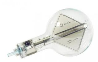
Tube allowing the study of electronic trajectories in electric and magnetic fields. A fluorescent screen with scale, inclined by  $10^{\circ}$  with respect to the axis of the beam, makes it possible to see the shape of the beam.
