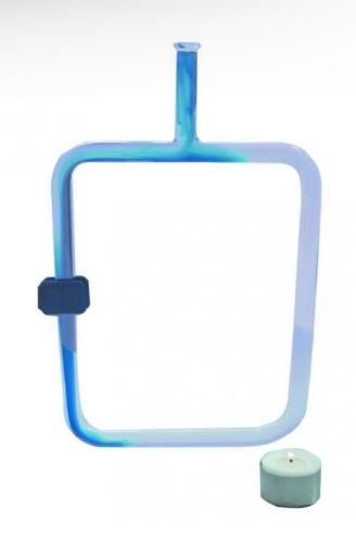
This glass tube makes it possible to visualize the convective movement of a fluid. Fill the tube with water and pour a few drops of dye. Light a candle at an angle of the system and observe the dye flowing away from the heat source. Dimensions :  $15 \times 20$  cm
