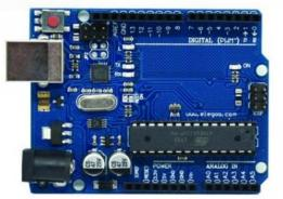
The Uno interface is based on the ATmega328 microcontroller.
