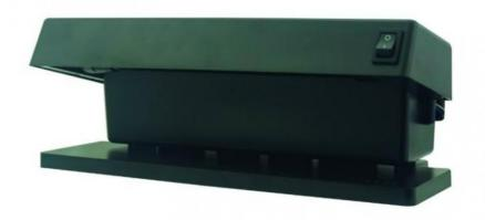
This lamp is composed of two UV tubes with a power of 6W and wavelengths 254 nm and 365 nm fixed under a protective housing. The lighting of the lamps is simultaneous (UVA + C at the same time). Integrated base.
