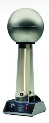
Van de Graaff apparatus generating very high voltages for electrostatic experiments. Sparks up to 100 mm can be obtained.
