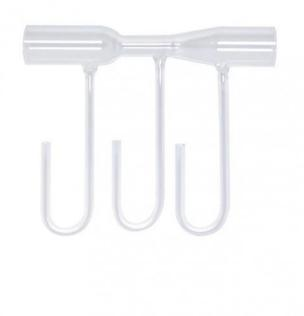
Venturi tube made of glass to view pressure differences near a constriction. 3 measuring points: before, after and at the level of the constriction
