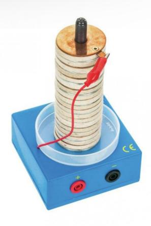
This product is a replica of the Alessandro Volta device: it is composed of galvanic cells connected in a series to constitute a source of electricity. Zinc and copper washers are stacked alternately onto each other and separated by a felt washer soaked in an electrolyte (salt or acid water) allowing the electricity to pass between the layers and thus measure the voltage between the two ends of this stack.
