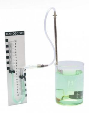
Manoscopic probe + water pressure gauge.
