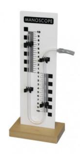
Water pressure gauge consisting of a U-tube fixed by 4 clips on a stand graduated in mm. At one end the reference pressure (atmospheric pressure) is applied and at the other end the pressure to be measured. The difference in liquid height corresponds to the pressure difference. Adjustment to zero is simply done by sliding the tube.
