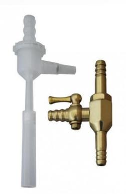
Assistent polypropylene water pump PP model with high chemical resistance. Safe use thanks to the incorporated non-return valve. R 3/4" union nut, E 1/2" reducer fitting and 10-12 mm olive screw connection Vacuum connection: olive screw Ø 6-9 mm, unscrewable with GL14 screw cap **Réf : TROMPA03**
