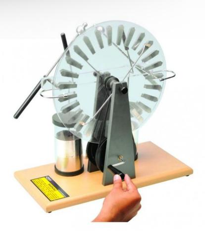
This machine made up of 2 transparent disks provided with metal segments, 2 capacitors (Leiden bottles), 2 discharge arms, and a plate makes it possible to carry out many experiments such as the study of the spark, its effects calorific and physiological, the distribution of charges, the lines of force of the electric field, etc.
