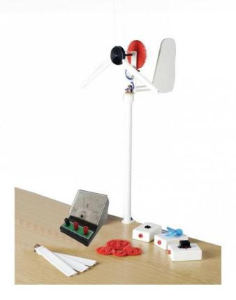
Complete kit to show the principle of operation of a wind turbine. The blades of the wind turbine are removable and adjustable.
