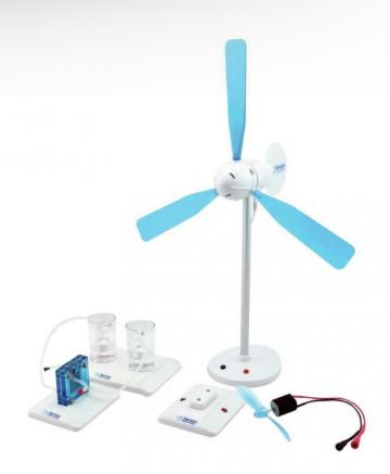
This set allows the transformation of wind energy into electrical energy through a reversible fuel cell. Included: Wind turbine on stand, fuel cell, hydrogen and oxygen tanks, motor with blades, 2 LEDs on stand, connection cords and accessories, assembly and operating instructions.
