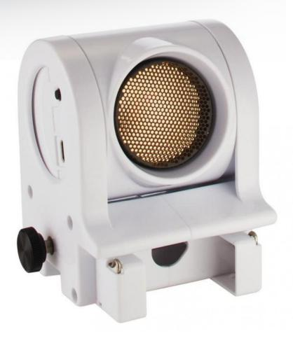
The wireless motion sensor measures the position, velocity and acceleration of objects using ultrasound. The wireless motion detector can detect objects within a radius of 15 cm to 4 m. Wireless sensor, ideal for applications at height (study of a fall...). The sensor connects directly to your devices via Bluetooth® or USB.
