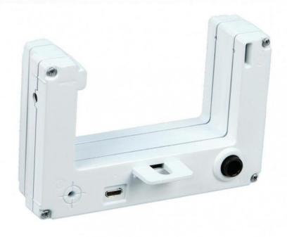
The most advanced WIRELESS PHOTOGATE to date! It has dual beams spaced 1.5 cm apart to accurately measure speed. The built-in laser switch allows you to time objects that are too large to pass through the WIRELESS SENSOR.
