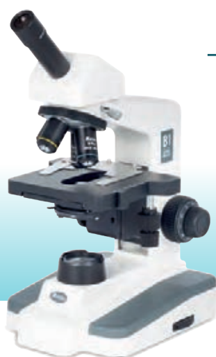
Microscope monoculaire MOTIC B1 Elite SP 4X/10X/40X
